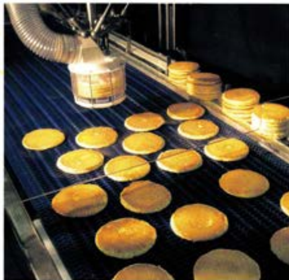
This stacking end effector loads entire stacks of pancakes.
